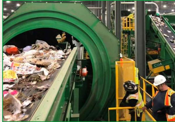
The waste is de-bagged, placed onto a conveyer then split into streams based on the size of the components. Items like textiles and large bulky items are separated out.
