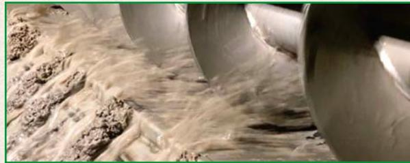
The remaining mixture of trash and paper are treated with water. Organic materials dissolve in the water and move on to step 7. The paper is broken down into pulp, which is the building block of new paper.
