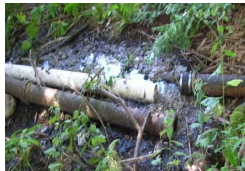
Failed PVC patch in private sewer line.
